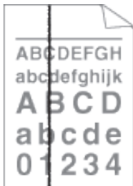
Black lines down the page Printed pages have toner stains down the page
