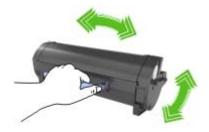
**5** Insert the toner cartridge into the printer by aligning the side rails of the cartridge with the arrows on the side rails inside the printer.
