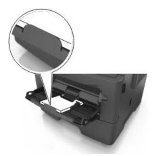
• Load letterhead faceup with the top edge entering the printer first. For two-sided (duplex) printing, load letterhead facedown with the bottom edge entering the printer first.
