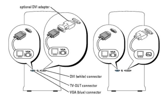
3. Make the appropriate connections for the second device that you are connecting.
