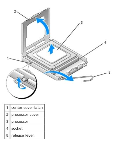
**NOTICE:** When replacing the processor, do not touch any of the pins inside the socket or allow any objects to fall on the pins in the socket.
