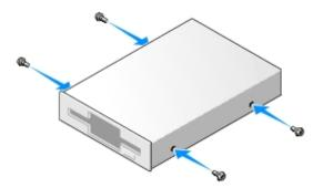
3. Align the shoulder screws on the floppy drive with the shoulder screw slots, and gently slide the drive into the bay until it clicks into place.
