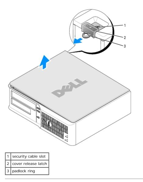
Removing the Computer Cover: Dell OptiPlex 320 User's Guide
