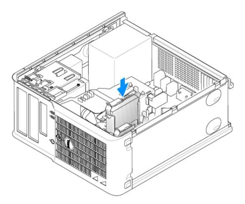
5. Connect the power and data cables to the drive.
