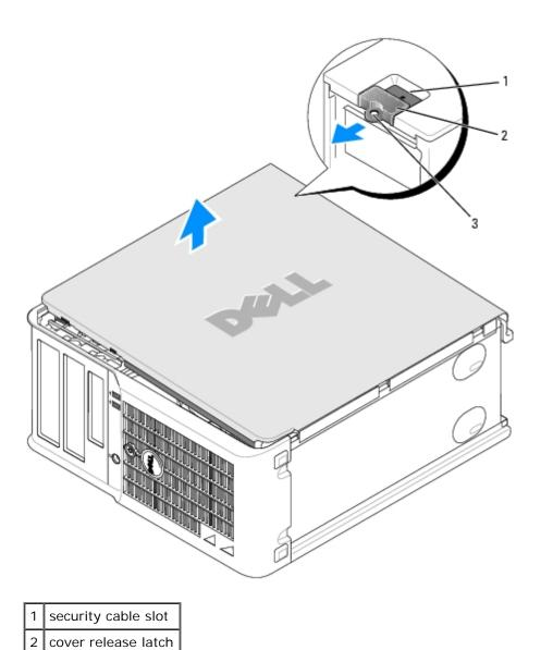
Removing the Computer Cover: Dell OptiPlex 320 User's Guide
