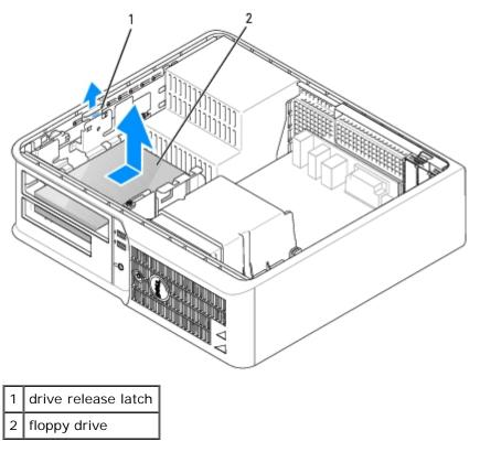
4. Disconnect the power and data cables from the back of the floppy drive.
