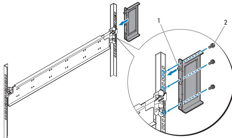
**4** Attach the right rail and stopping bracket to the rack.
