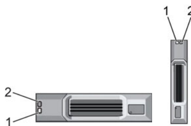
Figure 8. SCv300 and SCv320 Expansion Enclosure Drive Indicators
