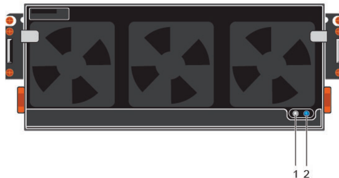
Figure 21. SCv360 Front-Panel Features and Indicators
