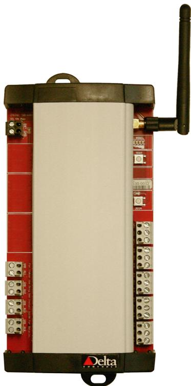
The eM-410R4 provides wireless remote I/O to a Wireless Coordinator. The controller has fixed algorithms that can be loaded in from the enteliTOUCH and configured to meet specific applications. The eM-410R4 also functions as a wireless repeater/router to extend the range of Delta enteliMESH devices.
