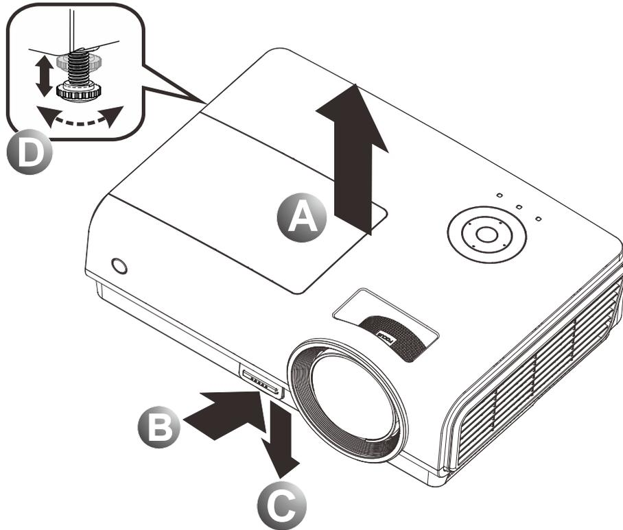
1. To raise the level of the projector, lift the projector [A] and press the height-adjuster button [B].
