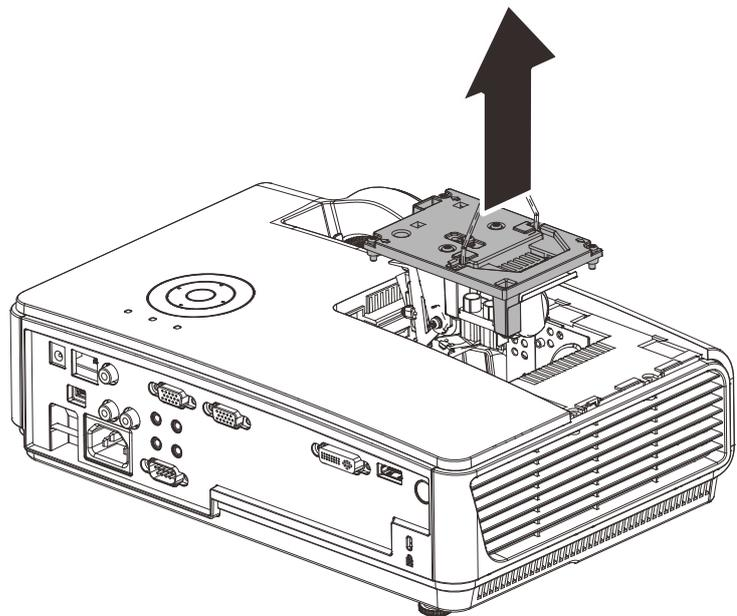
6. Reverse steps 1 to 5 to install the new lamp module. While installing, align the lamp module with the connector and ensure it is level to avoid damage.
