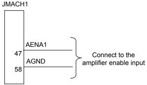
This signal could be either sinking or sourcing as determined by chips U37. (See jumpers E100-E102.) For 24V operation, E100 must connect pins 2-3 and a separate power supply must be brought on pins 9-7 of the J9 JEQU connector. The polarity of the signal is controlled by jumpers E17A to E17D. The default is low-true (conducting) enable. In addition, the amplifier enable signal could be controlled manually by setting Ix00=0 and using the suggested definition of the Mx14 variable.
