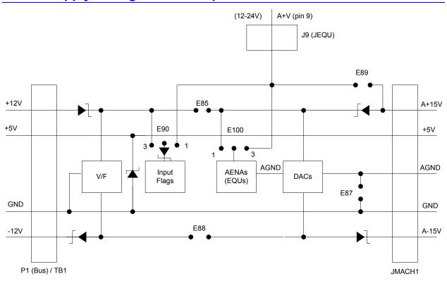
**E85, E87, E88:** Analog Circuit Isolation Control – These jumpers control whether the analog circuitry on the PMAC is isolated from the digital circuitry, or electrically tied to it. In the default configuration, these jumpers are off, keeping the circuits isolated from each other (provided separate isolated supplies are used).
