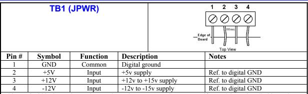
This terminal block may be used as an alternative power supply connector if PMAC is not installed in a PCI-bus. The +5V powers the digital electronics. The +12V and -12V (if jumpers E85, E87, and E88 are installed) power the analog output stage. This defeats the optical isolation on PMAC.
