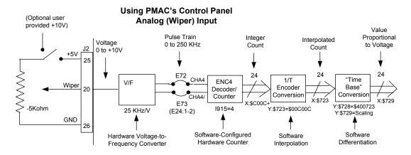
To use this value for feedrate override for a coordinate system, set the time base source address I-Variable (Ix93 for C.S.x.) to 1833 (\$729). To use this value for some other purpose, assign an M-Variable to this register (e.g., M60->X:\$729,0-24-,U). Scaling is set by the value in Y:\$729 (for the default conversion table). This value can be determined interactively by varying the input voltage and noting the effect.
