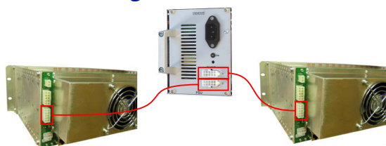
Backup Power for Two Master Units
