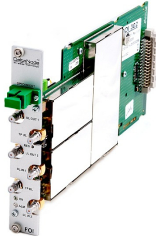
Figure 6 Fiber Optic Interface (FOI) Unit
