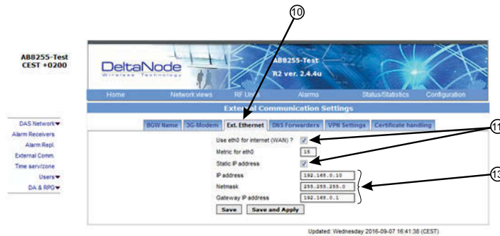
Figure 126 BGW Configuration - External Ethernet Setting
