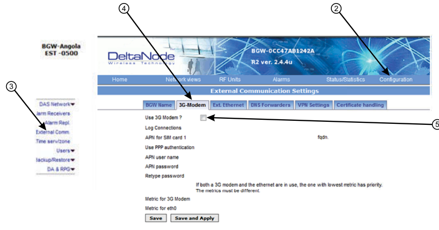
Figure 123 BGW Configuration - 3G Modem Setup
