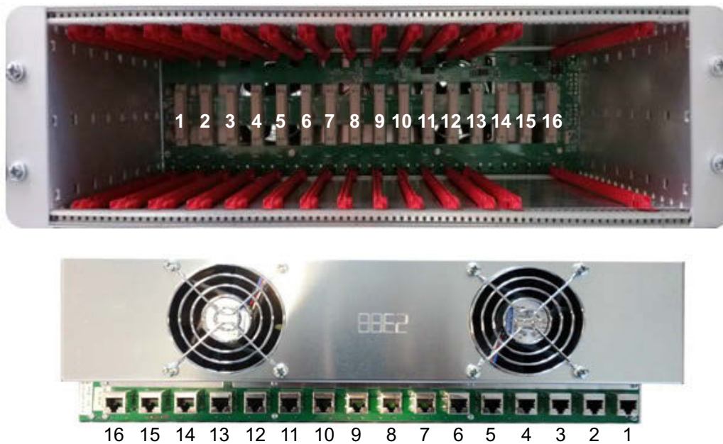
Figure 29 Ethernet Port Numbering, Front and Rear Views
