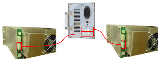
Backup Power for Two Master Units
