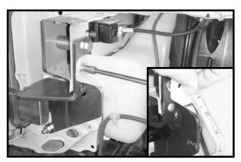
13. Reinstall windshield washer tank using two of the three previously removed bolts. Where washer tank lays on base plate, use enclosed 6mm-1.00 x 25mm bolt, 1/4" lock washer, and 1/4" flat washer to fasten. NOTE: On some models, it maybe necessary to trim mounting tab as shown in picture to clear base plate.
