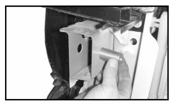
Slide spacer bushing into large hole in frame, on each side, from inside of frame outwards.
