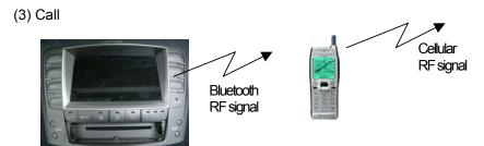
Call by inputting the phone number with the touch sensitive panel installed in the navigation system. Get the phone by operating the touch sensitive panel installed in the navigation system.
