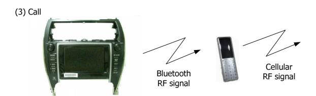
Call by inputting the phone number with the touch panel of the navigation system. Get the phone by operating the touch panel of the navigation system.
