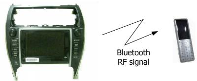
Transmits the selection signal from the navigation system to the Bluetooth product and connect the navigation system with the Bluetooth product.
