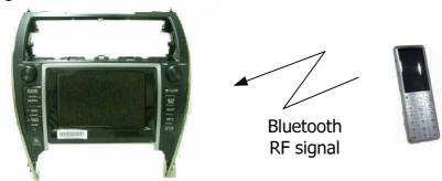
Transmits the registration signal from the Bluetooth product to the navigation system and register the Bluetooth product at the navigation system.
