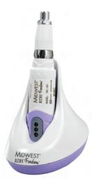
11.5 Invert the inner module and place it on the charging base as shown. The LED shown below will blink green if the position is correct for synchroni-
