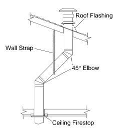
Figure 20 - Offset with Wall Strap and 45° Elbows
