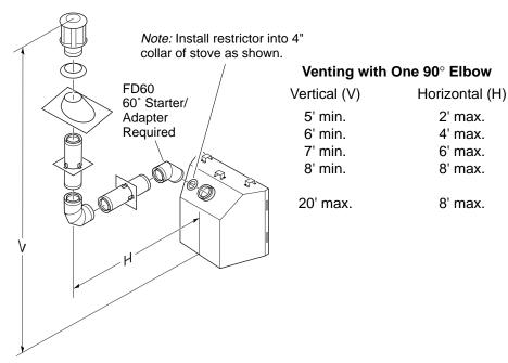
Figure 25 - Vertical Rigid Venting Configuration Using One 90° Elbow
