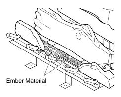
Figure 55 - Placing Ember Material on Burner
