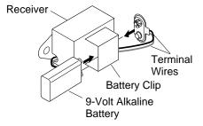
Figure 39 - Attaching Alkaline Battery to Receiver
