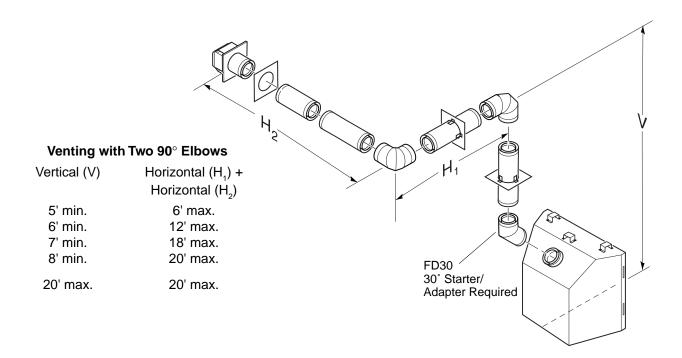
Figure 19 - Horizontal Termination Configuration for Rigid Venting Using Two 90° Elbows with Termination at 90° with Fireplace
