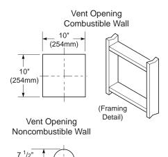
Figure 12 - Vent Opening Requirements
