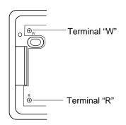
Figure 46 - Thermostat Base Terminals "W" and "R"
