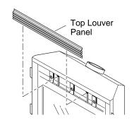
Figure 47 - Removing Top Louver Panel
