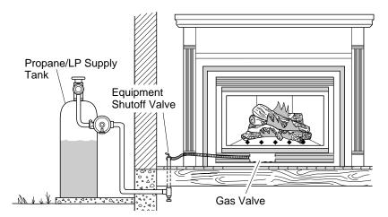
Figure 37 - Checking Gas Joints for Propane/LP Gas Fireplace
