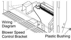
Figure 32 - Installing Plastic Bushing and Wiring Diagram Sticker
