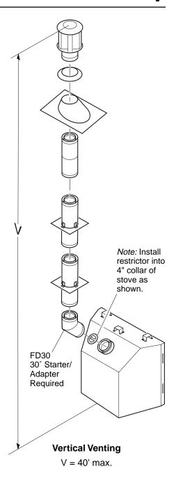
Figure 27 - Vertical Rigid Venting Configuration With No Horizontal Run
