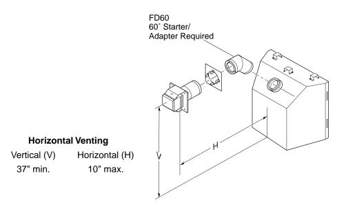
Figure 16 - Horizontal Termination Configuration for Rigid Venting
