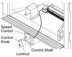
Figure 31 - Attaching Speed Control to Firebox
