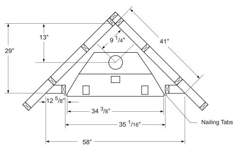
Figure 6 - Framing Clearances for Corner Installation
