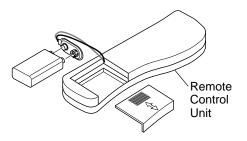
Figure 43 - Installing Battery in Hand-Held Remote Control Unit (GHRCTA Series Only)
