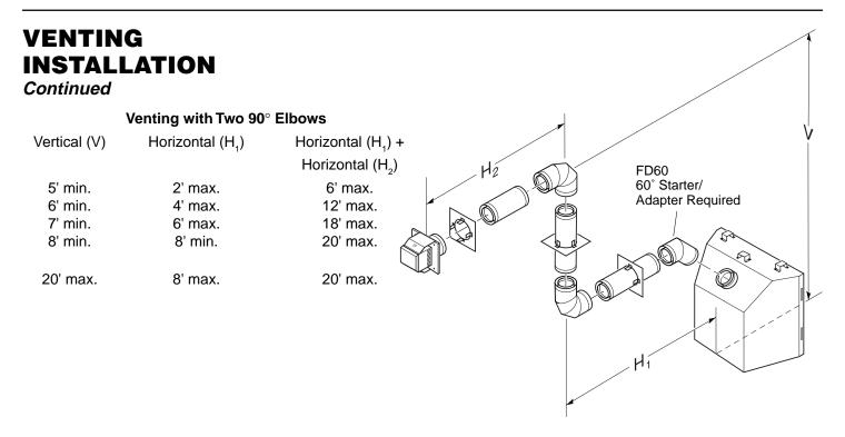
Figure 18 - Horizontal Termination Configuration for Rigid Venting Using Two 90° Elbows
