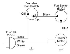
Figure 61 - Blower Wiring Diagram for Thermostat-Controlled Models
