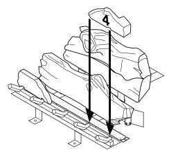
Figure 54 - Installing Log No. 4
