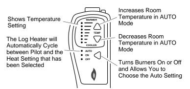
Figure 58 - Thermostat Hand-Held Remote Control Unit Selections (GHRCTA Series Only)
