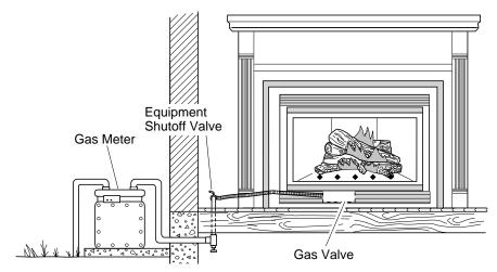
Figure 38 - Checking Gas Joints for Natural Gas Fireplace
