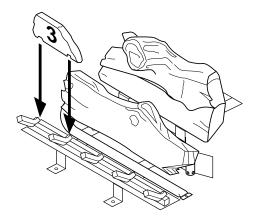
Figure 53 - Installing Log No. 3
