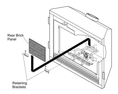
Figure 49 - Installing Rear Brick Panel and Retainer Brackets
