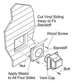
Figure 14-Installing Vinyl Siding Standoff
