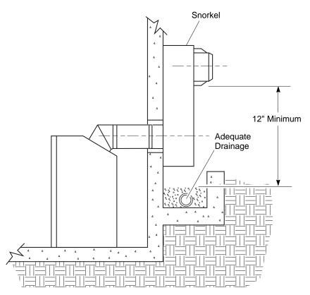
Figure 10 - Snorkel Termination with Drainage Pipe
