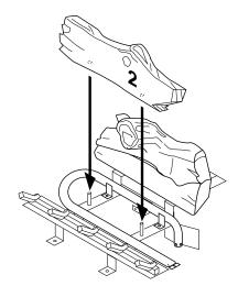
Figure 52 - Installing Log No. 2
