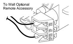
Figure 44 - Control Valve Terminals
