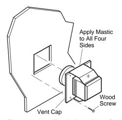
Figure 13 - Installing Horizontal Vent Cap
