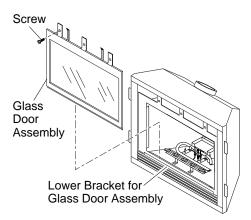
Figure 48-Removing/Replacing Glass Door
