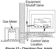
Figure 13 - Checking Gas Joints (Natural Gas Only)
