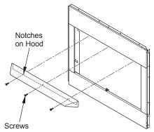
Figure 7 - Installing Hood
