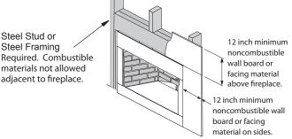
Figure 5 - Installing Firebox
