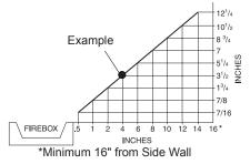
Figure 2 - Minimum Clearance for Combustible to Wall
