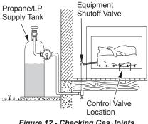
Figure 12 - Checking Gas Joints (Propane/LP Gas Only)
