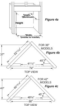
Figure 4 - Rough Opening for Installing in Wall
