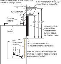
Figure 3 - Minimum Mantel Clearances for Built-In Installation
