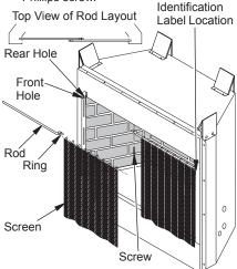
Figure 6 - Installing Fireplace Screen
