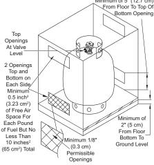
Figure 9 - Propane/LP Tank Enclosure
