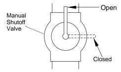
Figure 13 - Manual Shutoff Valve
