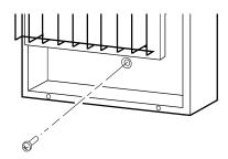
Figure 11 - Installing Bottom Mounting Screw
