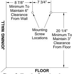
Figure 5 - Mounting Screw Locations
