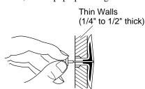
Figure 7 - Popping Open Anchor Wings For Thin Walls
