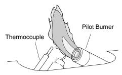
Figure 18 - Incorrect Pilot Flame Pattern
