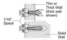
Figure 8 - Tightening Anchors
