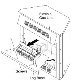
Figure 15 - Removing Fireplace Screen
