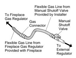
Figure 33 - Attaching Flexible Gas Lines Together
