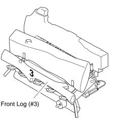
Figure 38 - Installing Front Log
