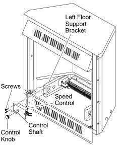
Figure 18 - Attaching Speed Control to Firebox
