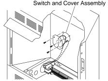
Figure 11 - Installing Switch and Cover Assembly
