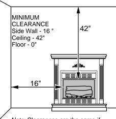
*Note:* Clearances are the same if using optional cabinet mantel or built-in installation.
