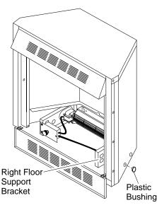
Figure 19 - Installing Plastic Bushing for Power Cord
