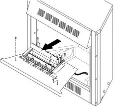
Figure 32 - Removing Log Base Assembly From Fireplace
