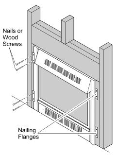
Figure 28 - Attaching Fireplace to Wall Studs Continued
