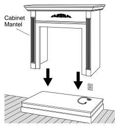
Figure 25 - Installing Cabinet Mantel
