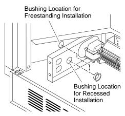
Figure 13 - Installing Bushings
