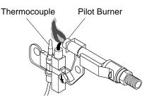
Figure 46 - Incorrect Pilot Flame Pattern
