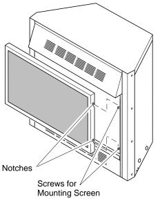
Figure 40 - Installing Fireplace Screen
