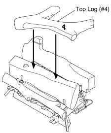
Figure 39 - Installing Top Log
