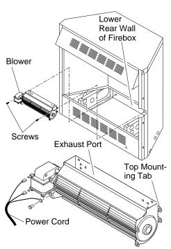
Figure 17 - Mounting Blower to Firebox
