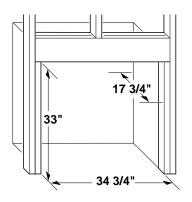
Figure 26 - Rough Opening for Installing in Wall
