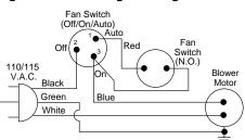
Figure 14 - Wiring Diagram
