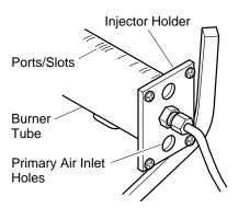
Figure 49 - Injector Holder On Outlet Burner Tube
