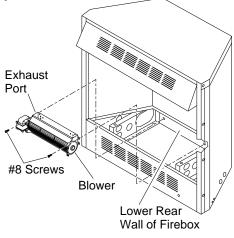
Figure 9 - Mounting Blower to Firebox
