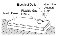
Figure 23 - Placing Hearth Base Accessory Against Wall
