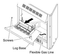
Figure 8 - Removing Log Base from Fireplace
