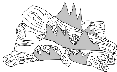
Figure 54 - Typical Flame Pattern for CHDV37N/P(A,B) and CHDV41N/P(A,B)
