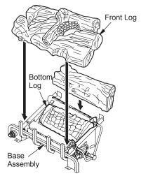
Figure 27 - Installing CRB and HRB Model Log Sets
