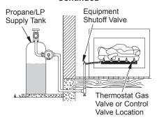
Figure 18 - Checking Gas Joints (Propane/LP Only)
