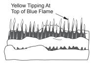
Figure 39 - Incorrect Front Burner Flame Pattern
