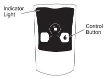
Figure 34 - On/Off Hand-Held Remote Control Unit
