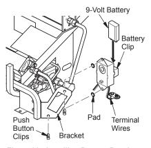
Figure 22 - Installing Remote Receiver
