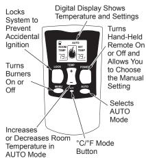
Figure 35 - Thermostat Hand-Held Remote Control Unit
