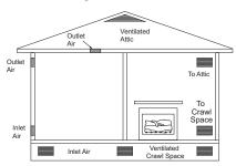
Figure 3 - Ventilation Air from Outdoors
