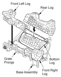
Figure 25 - Installing VUL Model Log Sets
