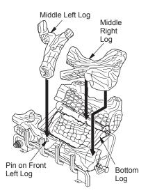
Figure 26 - Installing VUL Model Log Sets
