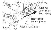
Figure 44 - Removing Thermostat Sensing Bulb
