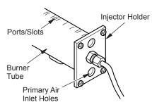
Figure 40 - Injector Holder On Outlet Burner Tube
