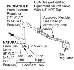
Figure 15 - Gas Connection (Thermostatically-Controlled Models Only)
