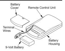
Figure 24 - Installing Battery in Hand-Held Remote Control Unit
