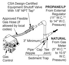
Figure 16 - Gas Connection (Remote-Ready Models Only)
