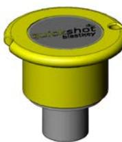
The Yellow Smart Key is used to initiate Centralised Blasting on a BCU connected to a Centralised Blasting Network. This is the only key that will be allowed to be inserted after a BCU is locked by the Surface Blast Controller. Note that a Surface Blast Controller lock that is issued from the controlling PC on surface is different to a detonator count lock, which is local to a particular BCU. No PIN is required for the Yellow key.
