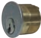
MC65 Mortise Cylinder - 1-1/8" 6-pin, keyed 5-pin. Available keyed alike or keyed differently. Finishes available: 605, 606, 612, 613, 626
