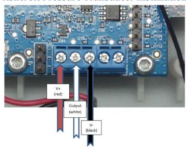
Bare wire (shield drain wire) from the transducer is unused.
