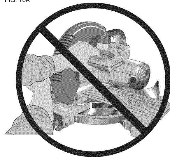
IMPROPER HAND POSITION
