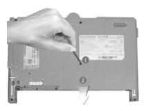
67 Slightly release two fasteners on SO-DIMM DDR module with your fingertip and take the module out.
