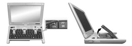
Gently move the keyboard forwards until the flat cable of keyboard is fully stretched, and then put the keyboard down on the top cover.
