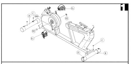
Remove the hex fixing bolts **(B)** from the front stabilizer **(A)** and rear stabilizer **(C)**. Align the holes in the main frame with the recessed nuts in the stabilizers and reinstall the fixing bolts.
