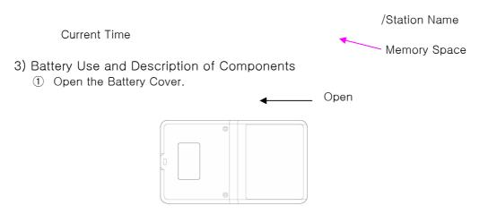
② Close the cover after inserting Rechargeable Li-Polymer Battery(3.7V/1500mAH) to the correct (+) (-) polarities.
