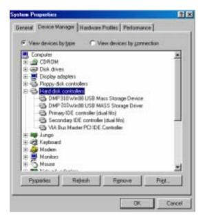
When installation is completed successfully, it is recognized as USB Mass Storage on Device Manager of My computer.
