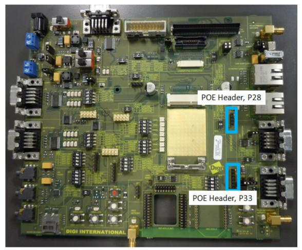
The development board provides two PoE module connectors, P28 and P33, to plug a Digi PoE module (DG-ACC-POE). The PoE module is an optional accessory item that can be plugged on the development board through the two connectors.
