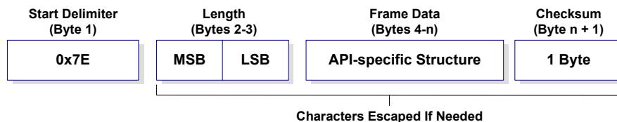
UART Data Frame Structure - with escape control characters:
