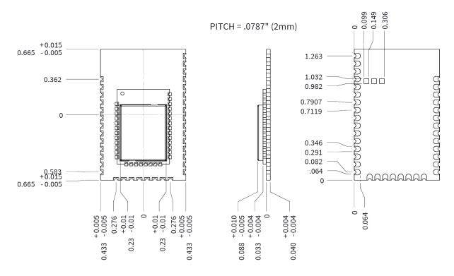
Mechanical drawings XBee3 micro antennas
