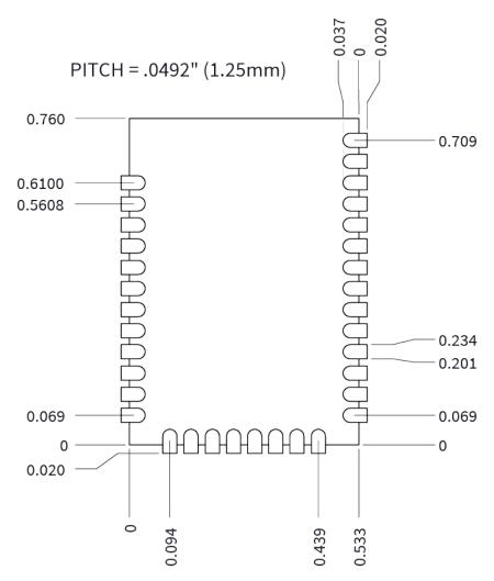
Match the solder footprint to the copper pads, but may need to be adjusted depending on the specific needs of assembly and product standards. Recommended stencil thickness is 0.15 mm/0.005". Place the component last and set the placement speed to the slowest setting.
