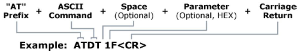
Figure 2-01. Syntax for sending AT Commands
