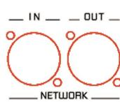
The network connections are established via two Neutrik™ EtherCon™ RJ45 receptacles. Connection is very easy: use the base labeled “IN” (“FROM”) to input the EtherSound stream, the base labeled “OUT” (“TO”) to send the EtherSound stream to other devices.
