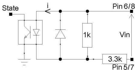
GPI #3 uses pins 5 & 6, GPI #4 uses pins 7 & 8.
