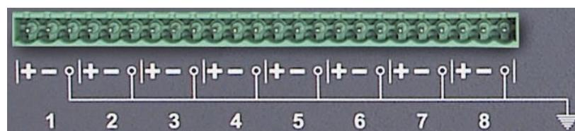
These balanced connections are compatible with unbalanced audio sources and destinations: just wire both cold pin and ground pin on ES8 to the ground of the unbalanced signal, and the ES8 hot pin to the signal.
