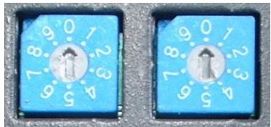
These two decimal rotary switches on the rear panel determine whether the assignment of the EtherSound channels to the analog inputs or outputs of ES8 is done locally or remotely by software control. The rotary switch on the left is the “tens” position and the rotary switch on the right is the “ones” position. Channels 1 to 64 are reserved for manual set-up, 0 and the channels from 65 on set the device to remote configuration mode.
