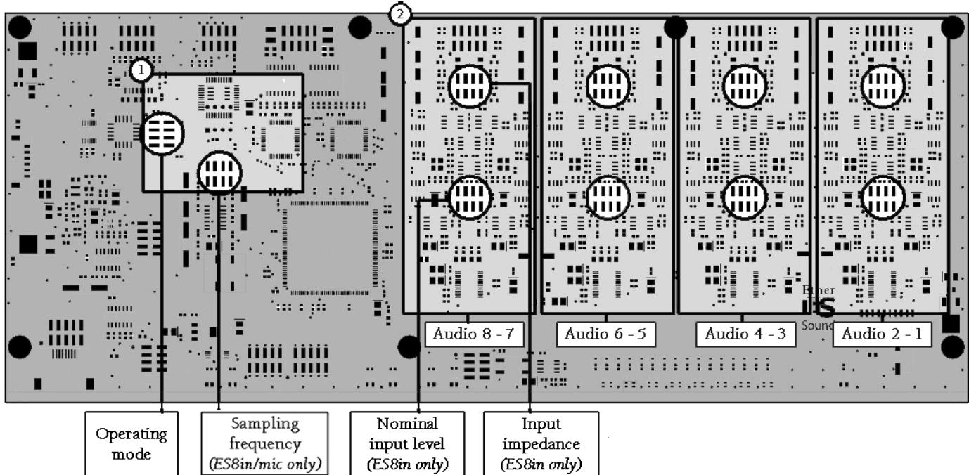
The figure above shows the locations of the different jumpers on the main board.
