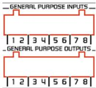
ES8in/ES8mic and ES8out feature four optocoupled GPIOs and four relay GPOs. GPIOs allow sending commands to the EtherSound configuration software, GPOs can be used by the EtherSound configuration software for remote control of external devices.
