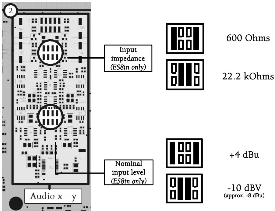
The settings described above relate to ES8in only, since they affect nominal input level and input impedance. Having located the pair to modify in the overview picture, set the jumpers according to the above illustrations to match the requirements of your system.
