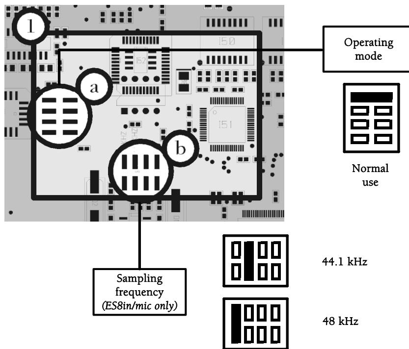
Section **a** shows the default setting for normal operating mode; this setting MUST NOT be modified. This jumper area is reserved for servicing purposes.
