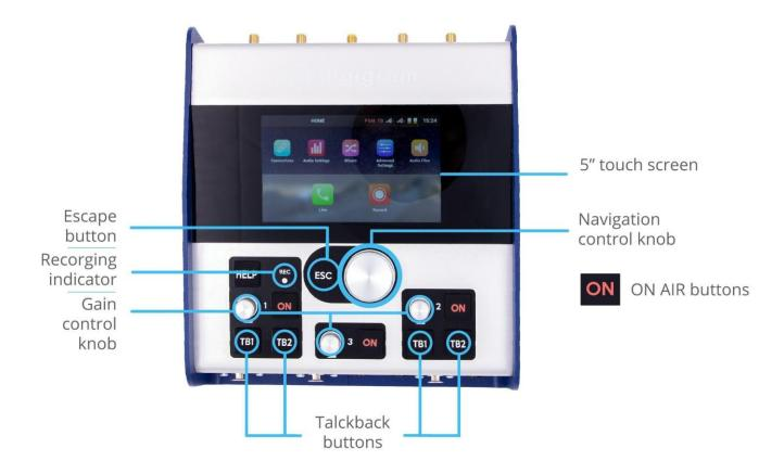
Push buttons and rotary knobs:
