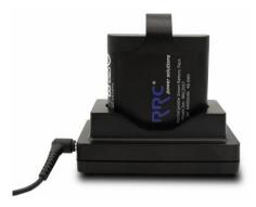
For the shipment of the product, the battery is put into "shipping" mode by the manufacturer. To enter "use" mode, the battery must first be placed in the external charger for a few hours (until the LED become green).
