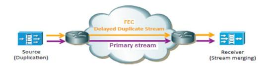
Multicast and unicast can be used for redundant dual streaming, and different UDP ports can also be used for the primary stream and the FEC stream.
