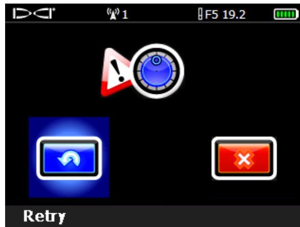
Roll Offset Failure Screen
