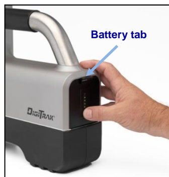
Battery Pack Fully Inserted
