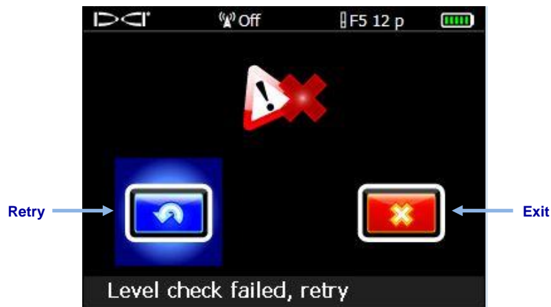
Level Test Failed Screen
