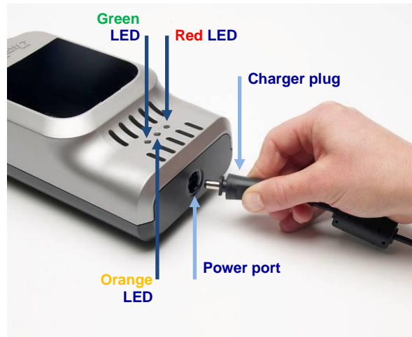
Inserting Charger Plug into Power Port
