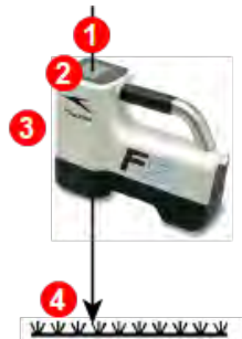
Plumb Line for Marking Locate Points
