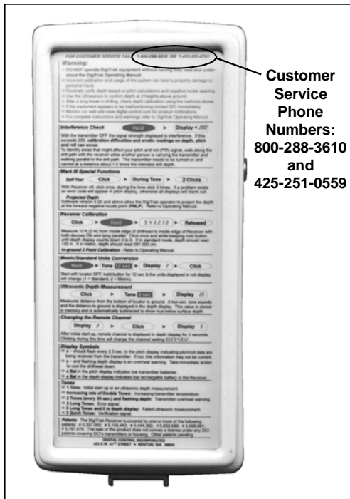
DigiTrak Receiver – Front Panel Showing Condensed Instructions
