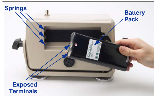
Installing Battery in Remote Display
