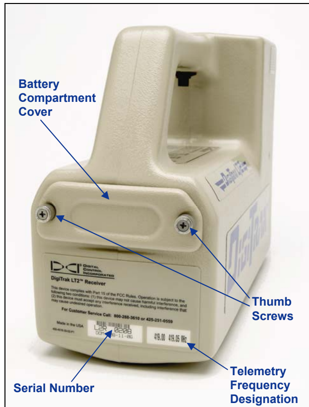
Back of Receiver Showing Serial Number and Telemetry Frequency Designation
