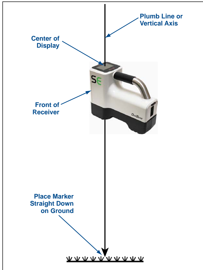
Plumb Line for Marking Locate Points
