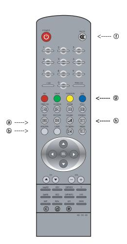
ⓐTEXT : Selects TELETEXT mode. See the page 24 in which the teletext function button is explained in detail.
