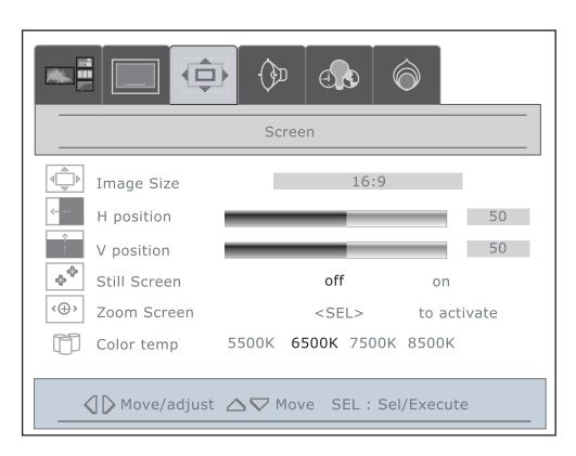
\* Color Temperature : The higher temperature, the cooler image is displayed.
