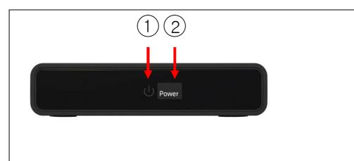
① LED : LED Lights up green when power is on. Lights up red when in Stand-By Mode.
