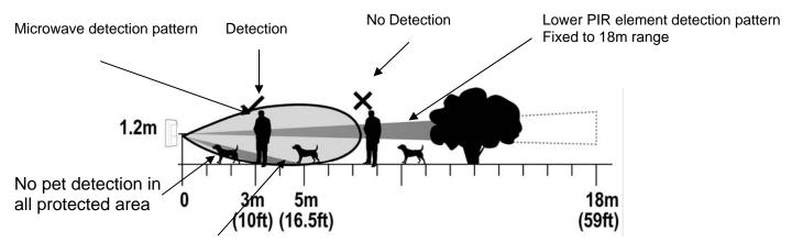
Upper PIR element detection pattern Adjustable between 3m and 18m (10 ft to 59 ft)
