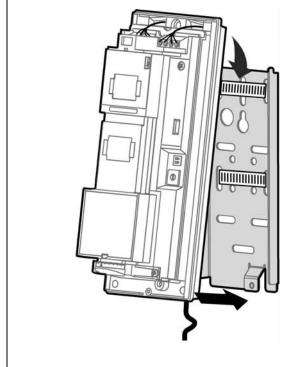
10. Attach the sealing "U" shaped Sponge Pad to the wire opening from the rear side after the wires have been connected and prior to final product affixing to the mounted bracket.
