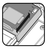
To adjust for ranges between 3m and 18m slide the detection element up or down to correspond with the desired distance. Each step between 3m and 18m represents 3m of range.
