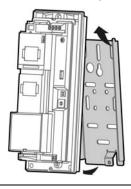
2. The detector is to be installed at height of 0.8 to 1.5 meter (ideally 1.2m)
