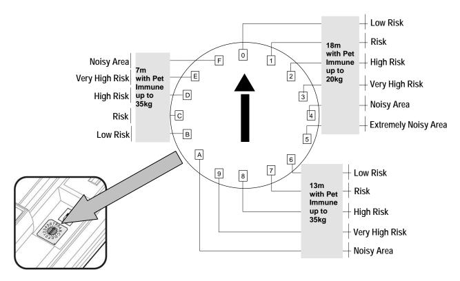
Each group is divided to 5 or 6 sub-positions that help to define the environmental condition inside the detection range:
