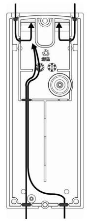
11. Place the detector on the mounting bracket from top side down and then lock the screw at the bottom.
