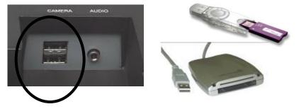
FIGURE 15 – CONNECTING A USB PERIPHERAL
