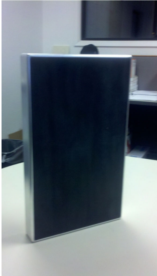
Duo-Sector Dual 5GHz 17dBi antenna
