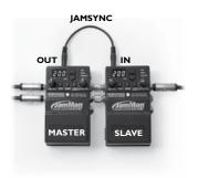
To use JamSync, connect the master JamMan Solo XT's JAMSYNC OUT jack to the JAMSYNC IN jack of the first slave device. Daisy chain any remaining JamSync slaves in the same manner.
