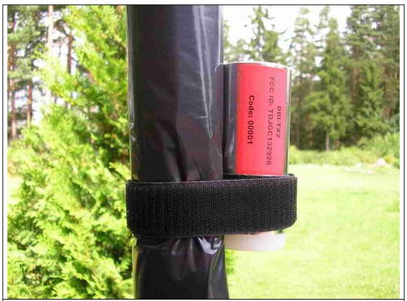
The DBI-TX2 attaches on one overhead frame rod. The IR lens aperture shall point straight up to the top centre of the envelope on a free line of sight.
